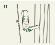
Make sure the lock works with your emergency keys before closing the door.
