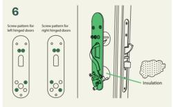
Locate the screw holes from the inside. Place the supplied insulation in both door holes. Mount the inside bracket with the cuttable screws. Tighten carefully. Two screws at the top and two at the bottom.
