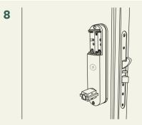
Insert the excess cord into the door to prevent it from getting caught. Slide the inside unit into place.
