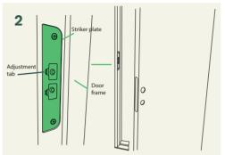
Mount the **striker plate** in your door frame, using the existing screws. If needed, you may readjust the adjustment tabs **after** the installation.
