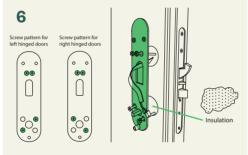
Locate the screw holes from the inside. Place the supplied insulation in both door holes. Mount the inside bracket with the cuttable screws. Tighten carefully. Two screws at the top and two at the bottom.
