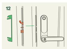
Close the door and verify that the hook bolt extends upon closure. If the gap between the door frame and door becomes too large, you can use the included spacer behind the strike plate.
