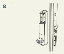
Insert the excess cord into the door to prevent it from getting caught. Slide the inside unit into place.
