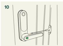
Mount both handles. The **exterior door handle** has a hole for the key cylinder. Place the handles in the desired direction and use the supplied tool to fasten the screws.
