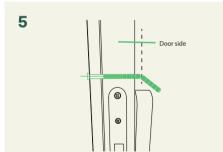
Adjust the **cuttable screws** so that they correspond to the thickness of the door and **add** an extra threaded portion. Use powerful pliers to cut to the desired length. The length should be equal on all screws. Cut further if necessary.
