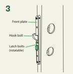
Verify that the **latch bolts** are set in the correct direction with the inclined side towards the doorframe. If necessary, remove the front plate and rotate the latch bolts. Mount the mortise in your door, using the existing screws.
