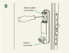
Fit the inside of the lock by fastening both the screws in the battery holder and the one at the bottom. Install all batteries and the battery cover.
