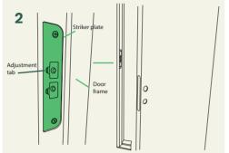
Mount the **striker plate** in your door frame, using the existing screws. If needed, you may readjust the adjustment tabs **after** the installation.
