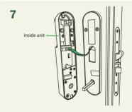
Place the rubber seal on the inner bracket and connect the **cable** to the inside unit.
