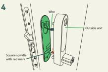
Place the **rubber seal** and the outside unit on the door. Make sure that the recessed area of the gasket is mounted towards the back of the lock. The red mark on the square spindle **must point up**. Pass the **wire** through the top.
